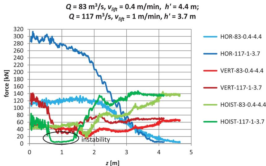
Figure 7. Examples of initially stable gate becoming temporarily unstable during lifting. Denotations in the legend: force (HOR, VERT, HOIST) [kN]– $Q$  [ $\text{m}^3/\text{s}$ ]– $v_{lift}$  [m/min]– $h'$  [m].
