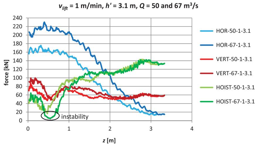
Figure 6. Examples of temporarily increased instability during the lift. Denotations in the legend: force (HOR, VERT, HOIST) [kN]– $Q$  [ $\text{m}^3/\text{s}$ ]– $v_{lift}$  [m/min]– $h'$  [m].
