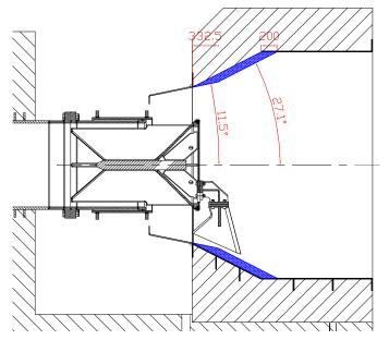
Fig.8: The longitudinal section of the final solution (in mm): The combination of LT 54, ring and hood modification.
