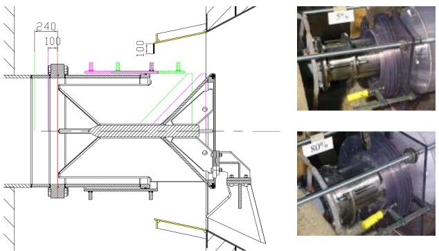
Fig.6: The lower half of the drawing shows the employment of the Litostroj's additional piece (LT 54) only, while the upper half shows the changed geometry due to the additional ring on LT 54; optimal position of the valve for s = 5 % opening is in green (photo top right), the optimal displacement of the valve for s = 80 % opening is in magenta (photo below).
