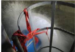
Fig.2: Back splash in the valve chamber.
