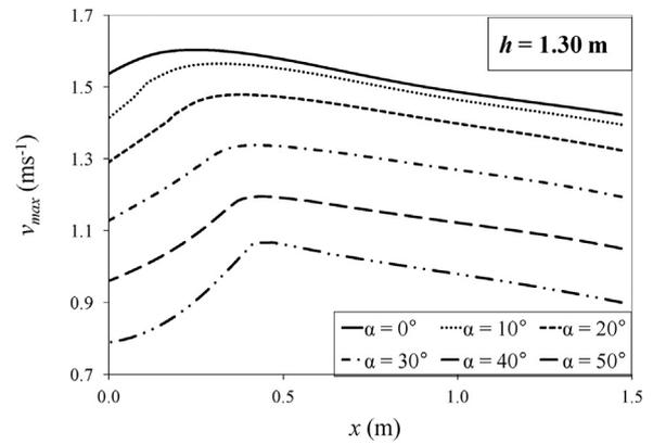
Fig. 12. Location of the profile with maximum velocity for  $h = 1.30$  m and  $b_0 = 0.59$  m.
