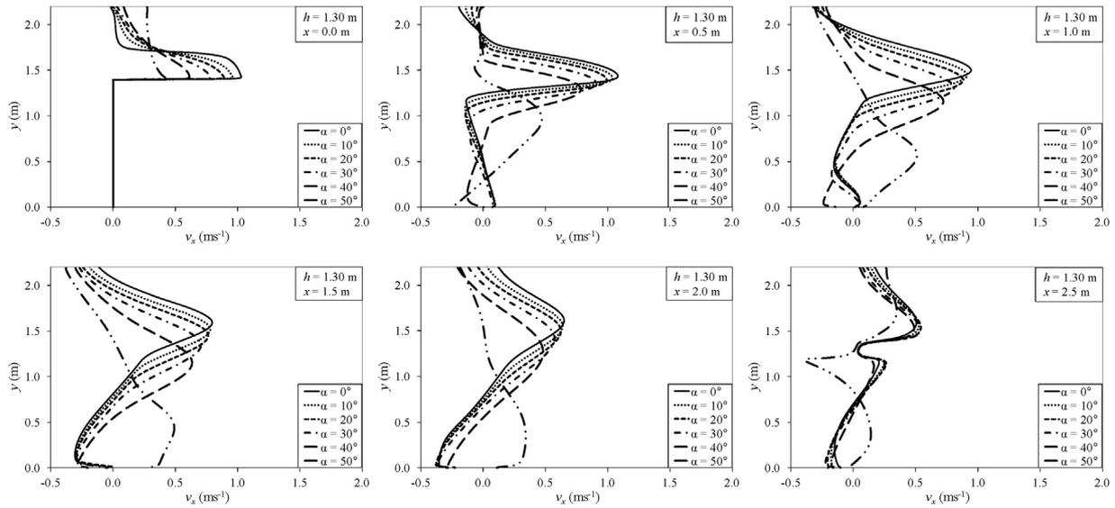
**Fig. 15.** Calculated longitudinal velocity components  $v_x$  at cross sections  $x = 0.5, 1.0, 1.5, 2.0$  and  $2.5$  m for geometries with slot width  $b_0 = 0.30$  m and different angle between baffles  $\alpha = 0^\circ, 10^\circ, 20^\circ, 30^\circ, 40^\circ$  and  $50^\circ$ .
