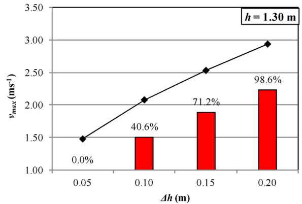
Fig. 19. Maximum velocities  $v_{max}$  at  $h = 1.30$  m,  $b_0 = 0.59$  m,  $\alpha = 20^\circ$  for  $\Delta h = 0.05, 0.10, 0.15$  and  $0.20$  m.
