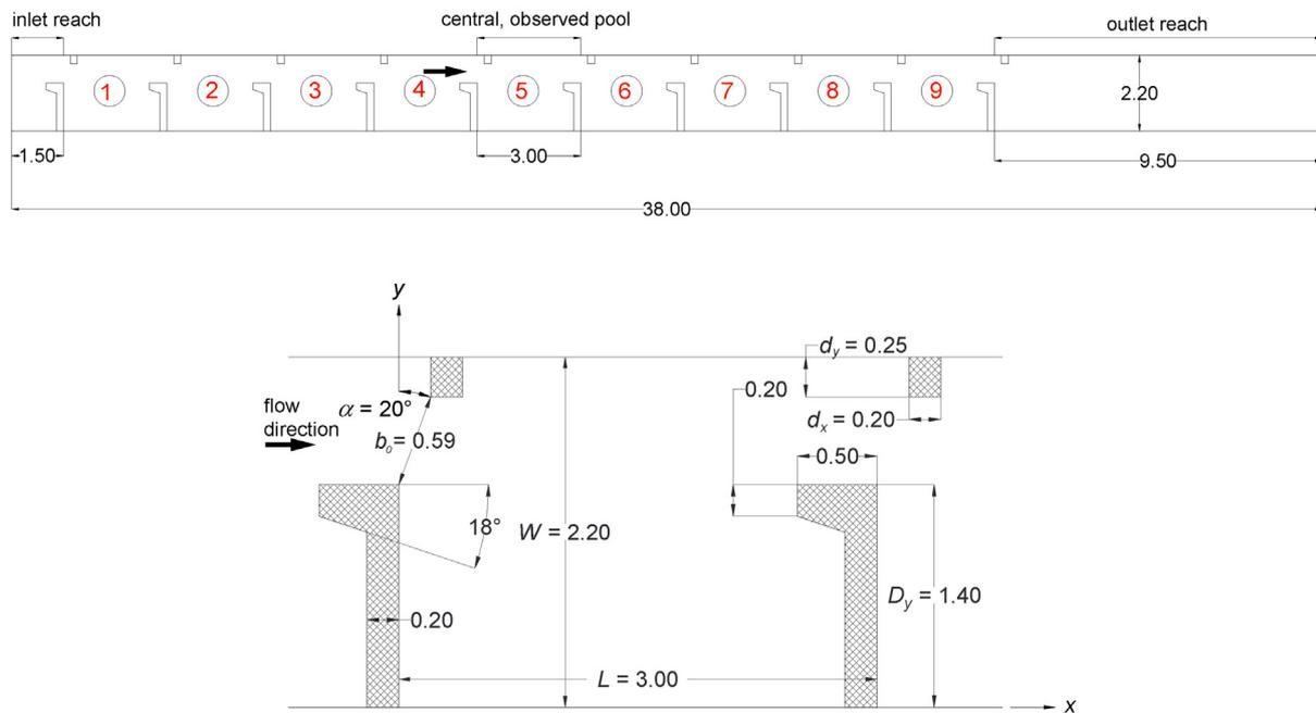
Fig. 1. Plan view of numerical model (above), details of a pool at the HPP Arto-Blanca (below). Dimensions are in meters.
