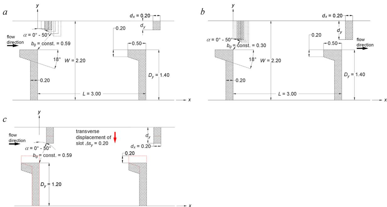
Fig. 2. Geometries of studied groups of variants: (2a) group of base geometries with slot width  $b_0 = 0.59$  m; (2b) group of geometries with smaller slot width  $b_0 = 0.30$  m; (2c) group of geometries with transverse displacement of the slot for  $\Delta s_y = 0.20$  m to the center of the pool and slot width  $b_0 = 0.59$  m. Dimensions are in meters.
