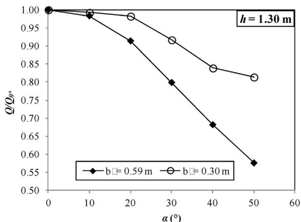
Fig. 7. Normalized discharge  $Q/Q_0$  (where  $Q_0$  means  $Q(\alpha=0^\circ)$ ) in relation to  $\alpha$ .
