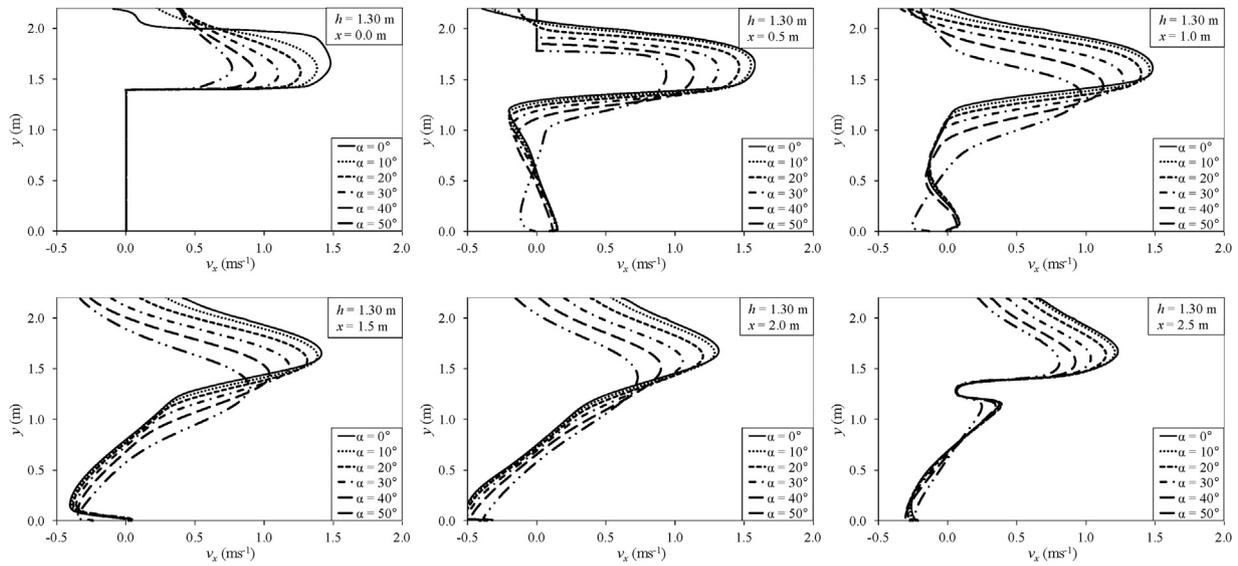
**Fig. 14.** Calculated longitudinal velocity components  $v_x$  at cross sections  $x = 0.5, 1.0, 1.5, 2.0$  and  $2.5$  m for geometries with slot width  $b_0 = 0.59$  m and different angle between baffles  $\alpha = 0^\circ, 10^\circ, 20^\circ, 30^\circ, 40^\circ$  and  $50^\circ$ .
