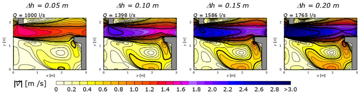
Fig. 20. Calculated isovels in the central pool of the VSF at  $h = 1.30$  m,  $b_0 = 0.59$  m,  $\alpha = 20^\circ$  for  $\Delta h = 0.05, 0.10, 0.15$  and  $0.20$  m.
