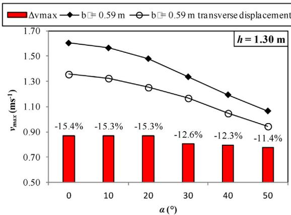
Fig. 17. Maximum velocities  $v_{max}$  for  $h = 1.30$  m and  $b_0 = 0.59$  m with various displacements of the slot.
