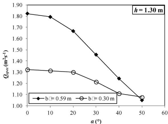
Fig. 9. Relation between discharge per unit width ( $Q_{\text{spec.}} = Q/b_0$ ) and  $\alpha$  for  $h=1.30$  m.
