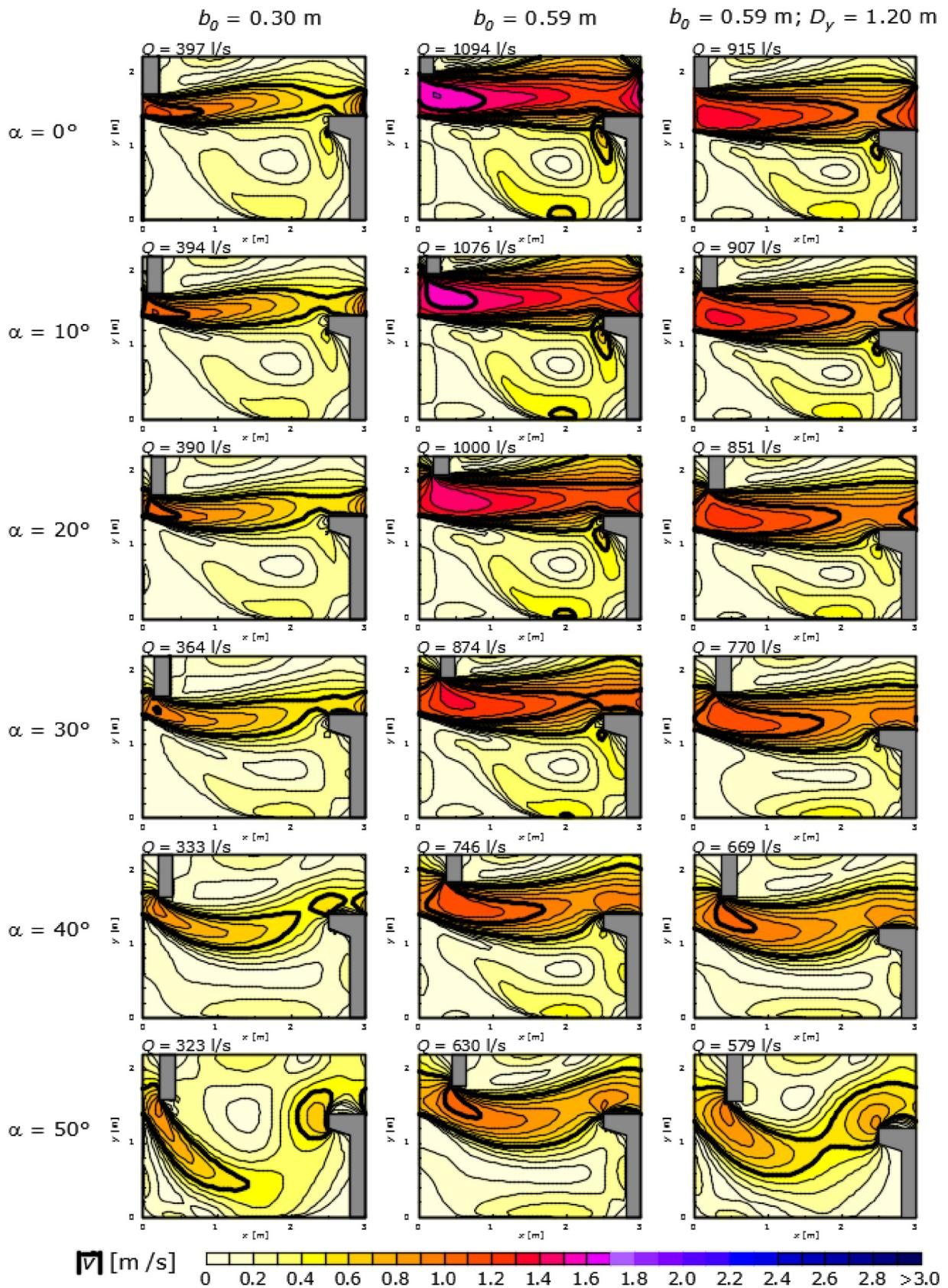
Fig. 13. Calculated isovels in the central pool of the VSF.
