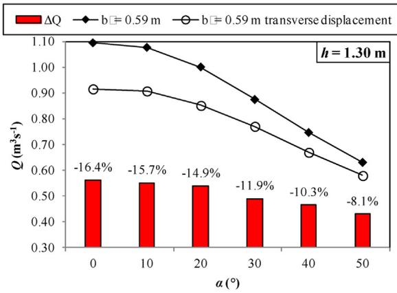
Fig. 16. Discharge at  $h = 1.30$  m and  $b_0 = 0.59$  m for different transverse positions of the slot.
