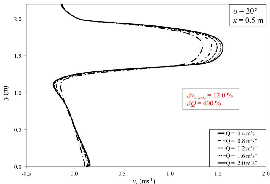
Fig. 6. Calculated longitudinal velocity components  $v_x$  at cross section  $x=0.5$  m for discharges  $Q=0.4, 0.8, 1.2, 1.6$  and  $2.0$   $\text{m}^3\text{s}^{-1}$  (case S1A2).
