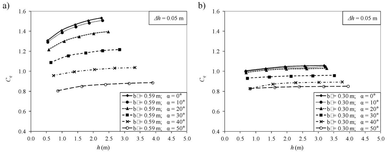
Fig. 4. Discharge coefficient  $C_q$  for cases with slot width  $b_0 = 0.59$  m (left) and for cases with slot width  $b_0 = 0.30$  m (right).
