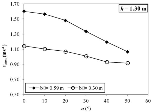
Fig. 10. Maximum velocity  $v_{max}$  of the flow with  $h = 1.30$  m for both openings  $b_0$  and various angles  $\alpha$ .
