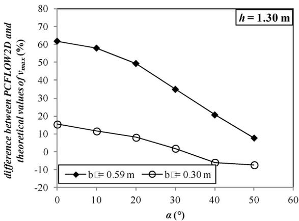
Fig. 11. Difference between PCFLOW2D and theoretical values of  $v_{max}$  at  $h = 1.30$  m.
