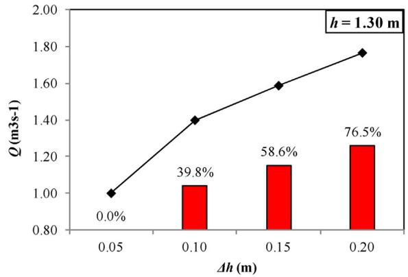
Fig. 18. Discharge at  $h = 1.30$  m,  $b_0 = 0.59$  m,  $\alpha = 20^\circ$  for  $\Delta h = 0.05, 0.10, 0.15$  and  $0.20$  m.
